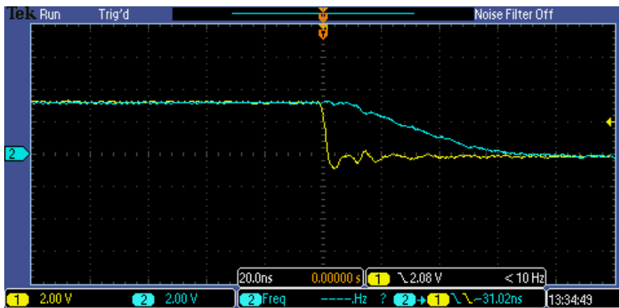
Figure 3.5: Slew rate difference between the LED pin (blue) and the SPD (yellow)
